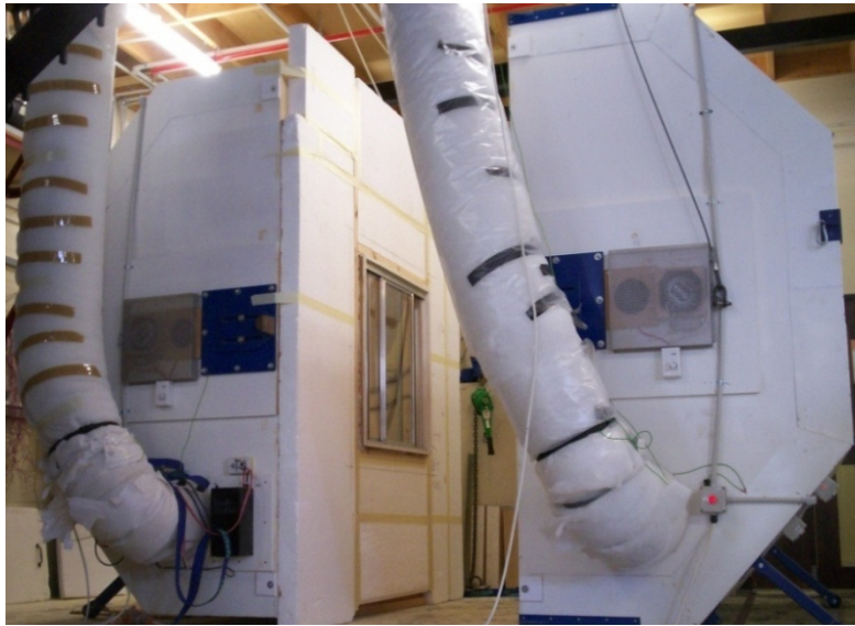
Fig. 1: The Guarded Hotbox Opened Between Tests
