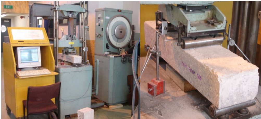
Figure 5 – Testing machine used to get the flexural tensile strength and displacement of the strips
