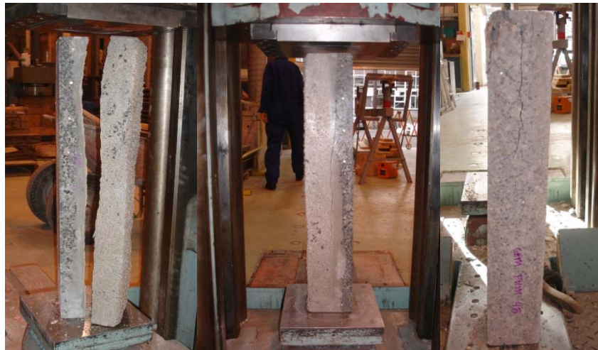
Figure 4 – Failure modes of stratified concrete loaded in compression
