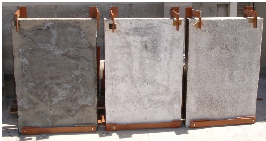
Figure 3 – Panels left exposed in outdoor conditions for 5 months
