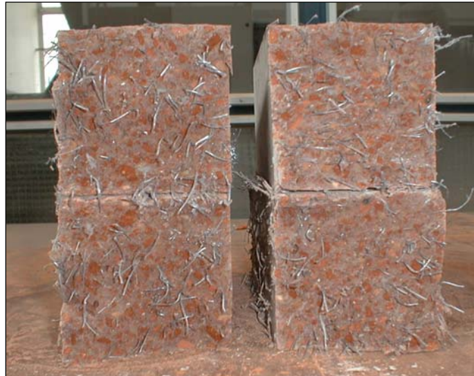
Figure 2: Specimens with recycled masonry aggregate
